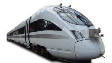
The Advanced TrainLab has a diesel-electric drive system, which enables test rides with a top speed of up to 200 km/h anywhere in DB's railway network. The 107 meter long train consists of 4 wagons, one equipped with the sensors and recording system of the CLUG project.
